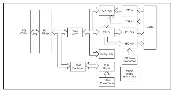
Figure 1-1. NI 8254R Block Diagram
